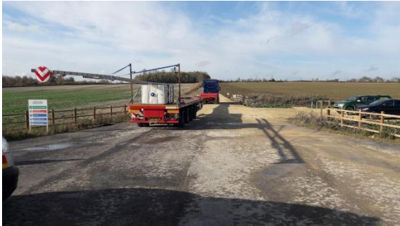
Wind turbine trial run enters site at the bell-mouth on the A1 and proceeds through the wind farm access tracks
